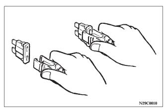
5. Insert a new fuse of the same capacity securely into the fuse block location.
